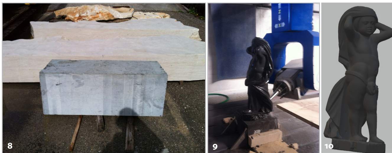
Figures 8, 9 y 10. - Figura 8: The limestone block of “preto ruço” before modelling. Figure 9: An aspect of the CNC during operations. Figure 10: Final result of the CNC machine operating process.
