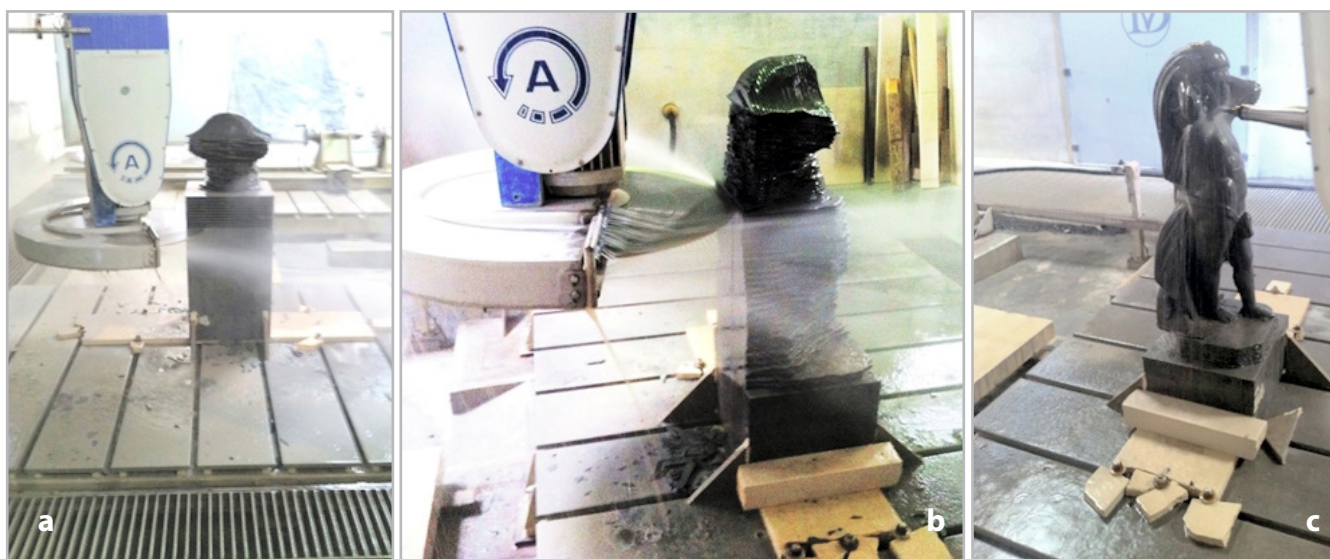
Figures 11 a, b, c. - Various stages of stone block cutting on a CNC machine
