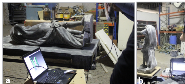
Figuras 6 a y b.- Structured light image capture from different sculpture positions.
